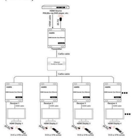
Connect HDMI Transmitter port and Receiver ports to the Ethernet Switch
